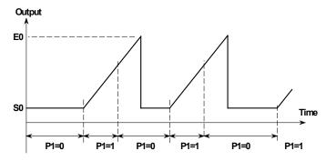
A **Frequency Sweep Dwell** only returns to the start value after a falling edge transition on the appropriate profile input
