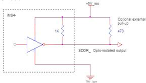
Diagram shown with optional external pull-up resistor to improve the rising edge on SDIO Bits 4..11 Min value 330ohm . Internally fitted on Bits 0..3
