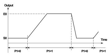
Both plots show a ramp on output J2, controlled using input P1 (on connector J8).
